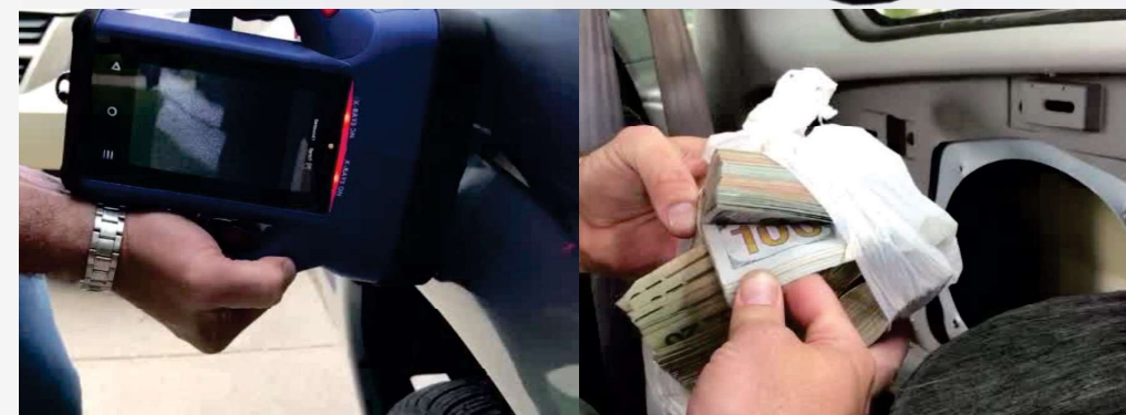
The HBI-120 revealed this hoard of cash hidden inside of a vehicle's quarter panel. The trim and speaker were then removed to retrieve it.
