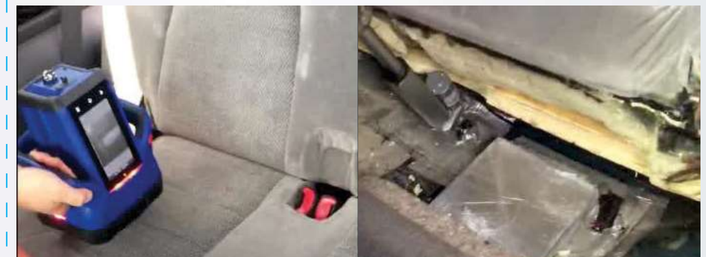
The HBI-120 revealed an anomaly beneath the seat of this vehicle. A kilo of marijuana was located in an engineered "trap" below the seat.
